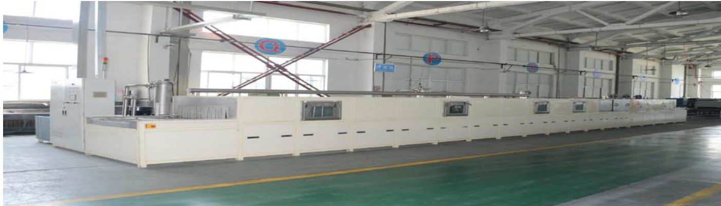
Automatic cleaning line
